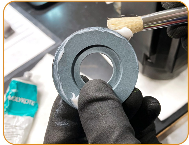
Figure 3-5: MOLYKOTE grease to coat the outer diameter O-ring
